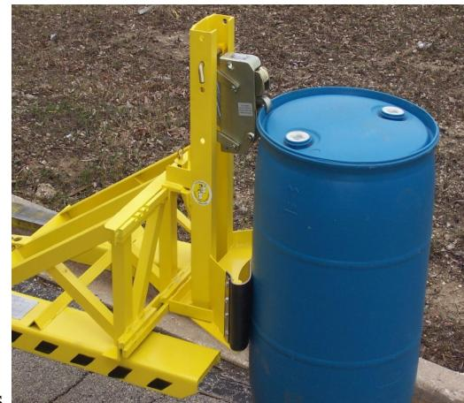
securely engage each drum in one place on the top chime offering an effective grip on every drum! This product is ideal for routine handling and transportation of drums on smooth warehouse floors, loading and unloading drums from pallets, or staging product for shipment. Cushioned belt-cradles on all FTA units protect the drum's sidewall during the pick-up and transport process.
